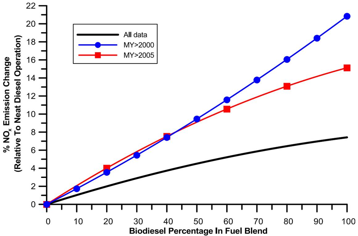
**Fig. 15** – Comparative NO<sub>x</sub> emission change best-fit curves for various engine model years.
