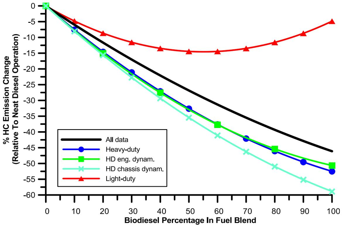
**Fig. 12** – Comparative HC emission change best-fit curves for various transient cycles and engine types.
