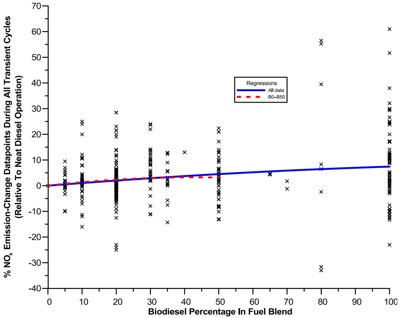
**Fig. 5** – NO<sub>x</sub> emission-change datapoints and best-fit curve when using various biodiesel-diesel blends during all transient cycles.
