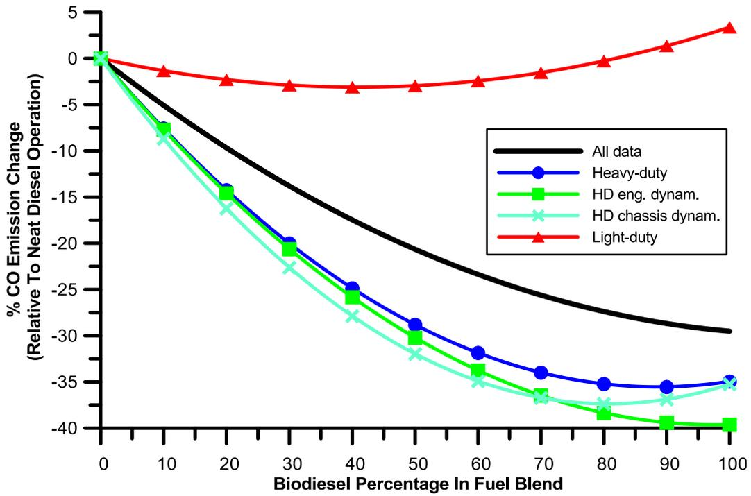
**Fig. 11** – Comparative CO emission change best-fit curves for various transient cycles and engine types.
