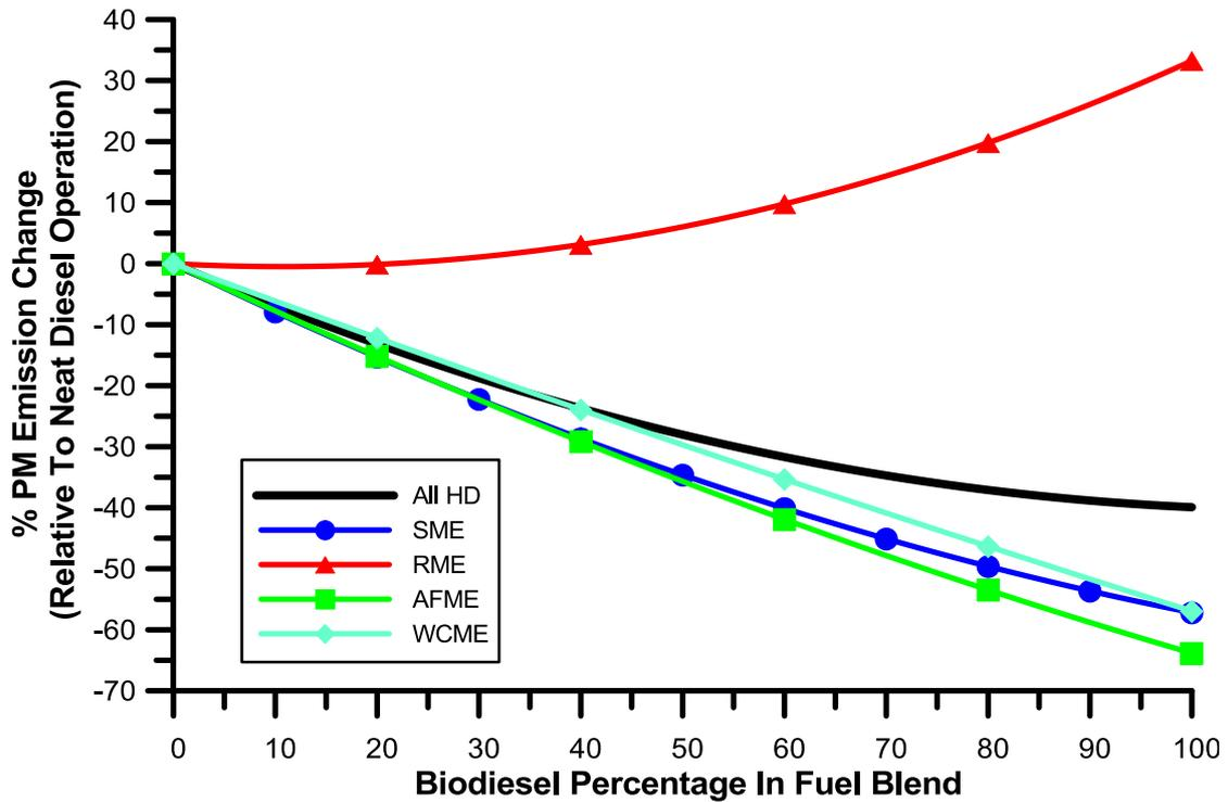
**Fig. 21** – Comparative PM emission change best-fit curves for HD engines and for various biodiesel feedstocks.
