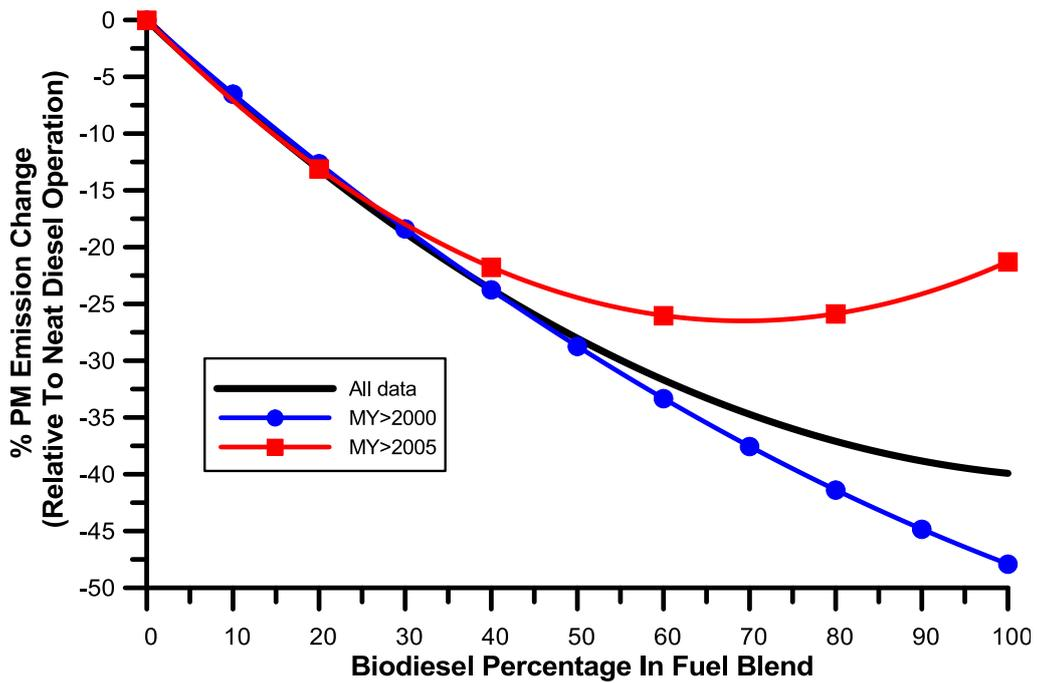
**Fig. 14** – Comparative PM emission change best-fit curves for various engine model years.
