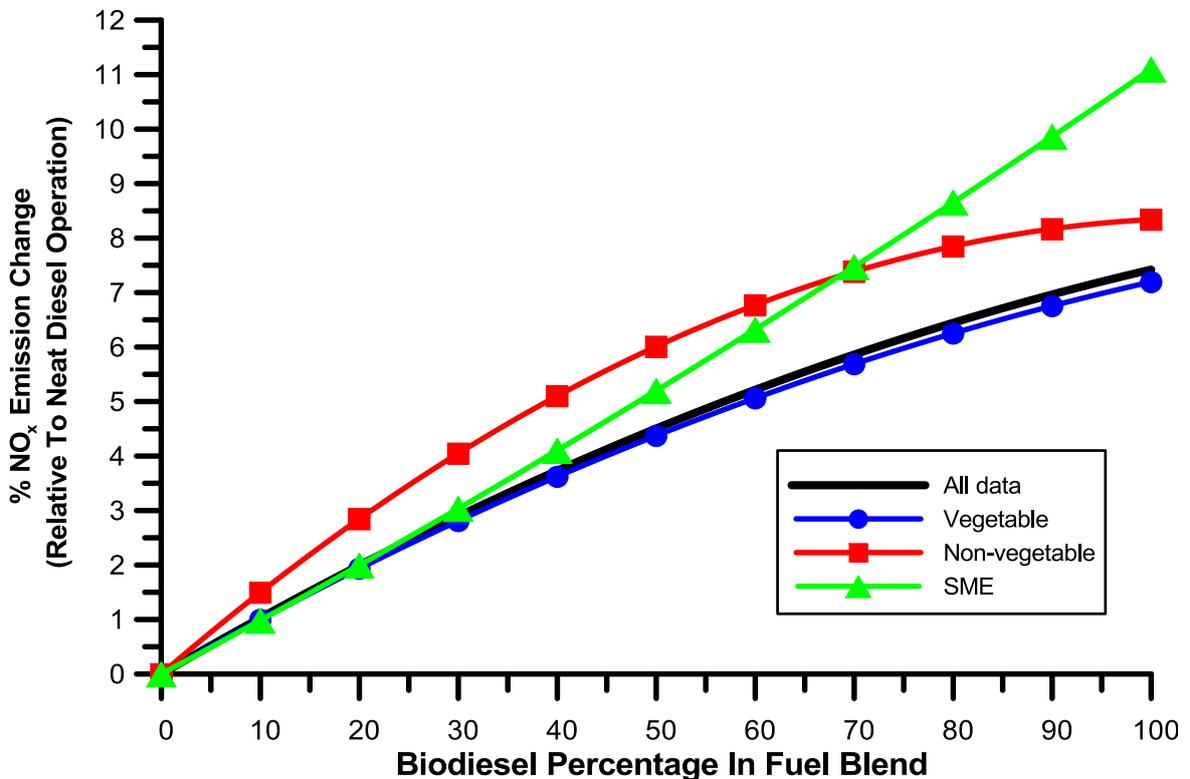
**Fig. 20** – Comparative NO<sub>x</sub> emission change best-fit curves for various biodiesel feedstocks.
