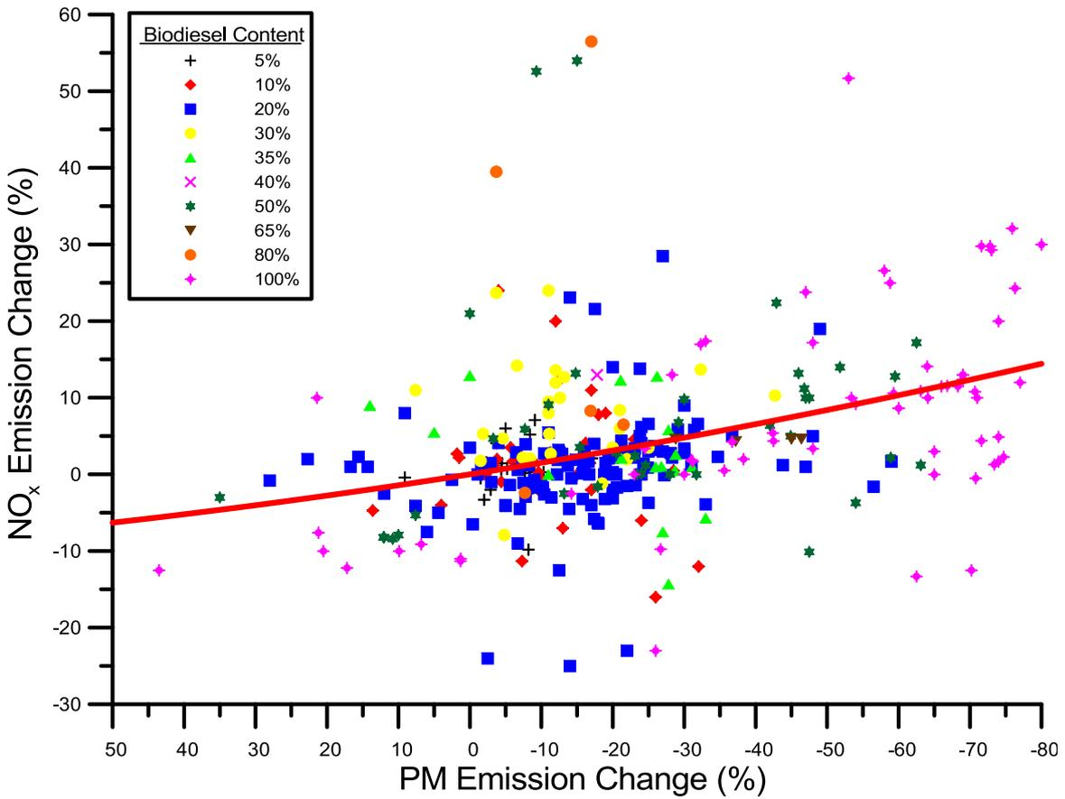
**Fig. 24** – Collective PM/NO<sub>x</sub> trade-off from all biodiesel blend ratios and transient cycles.
