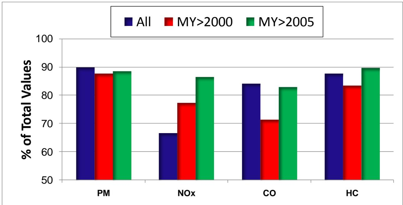
**Fig. 18** – Percentage of total negative (PM, CO, HC) or positive (NO<sub>x</sub>) measurement values for engine model year.
