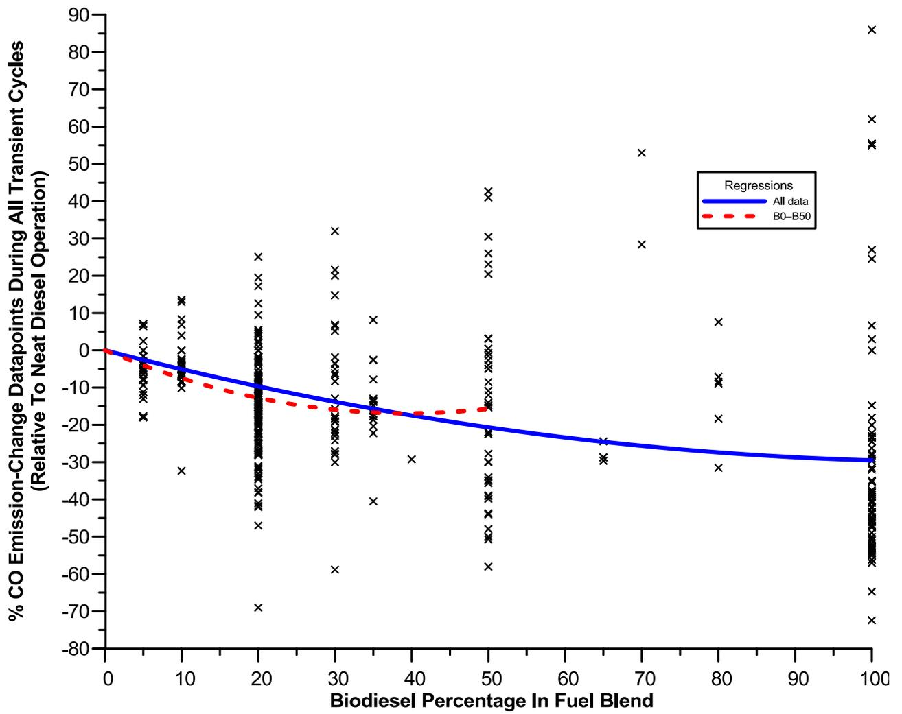
**Fig. 6** – CO emission-change datapoints and best-fit curve when using various biodiesel-diesel blends during all transient cycles.
