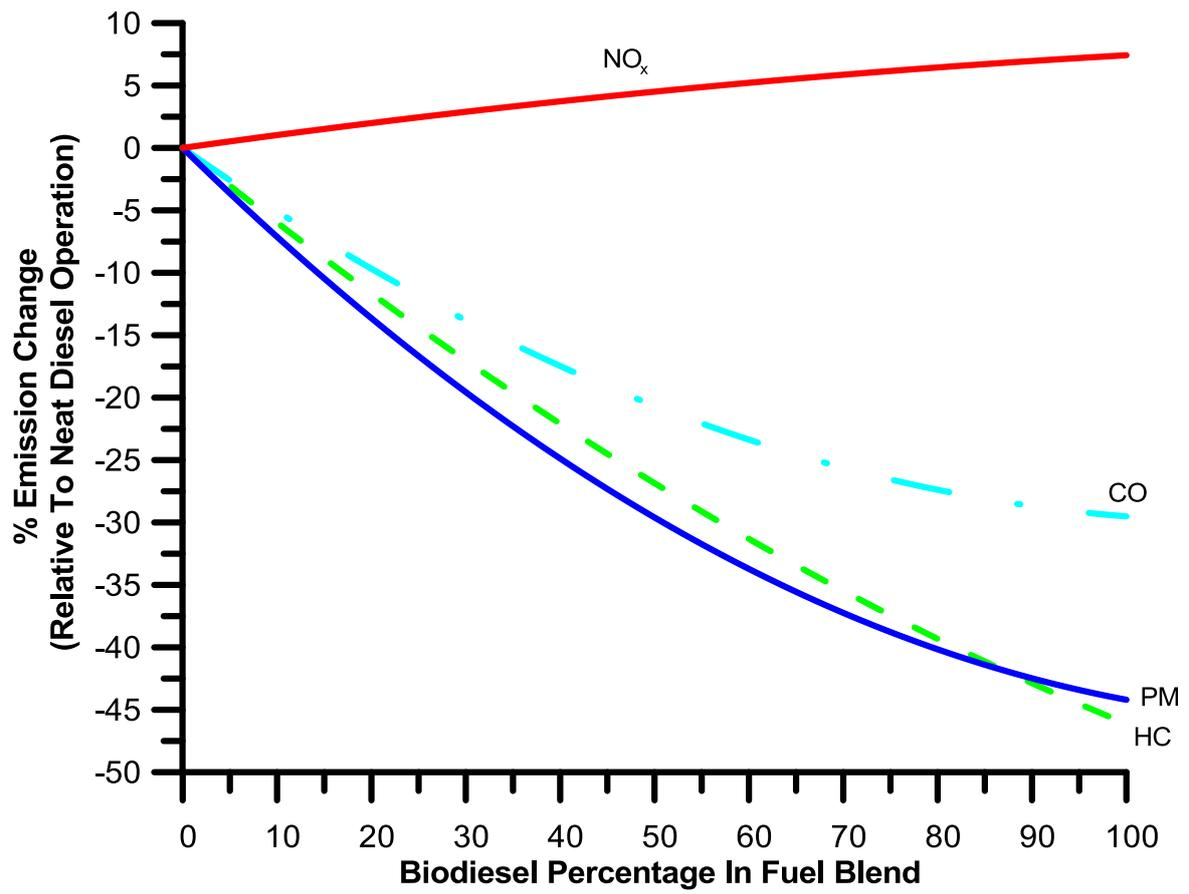
**Fig. 25** – Collective results of biodiesel effects on regulated pollutants from all transient cycles up to 2011.
