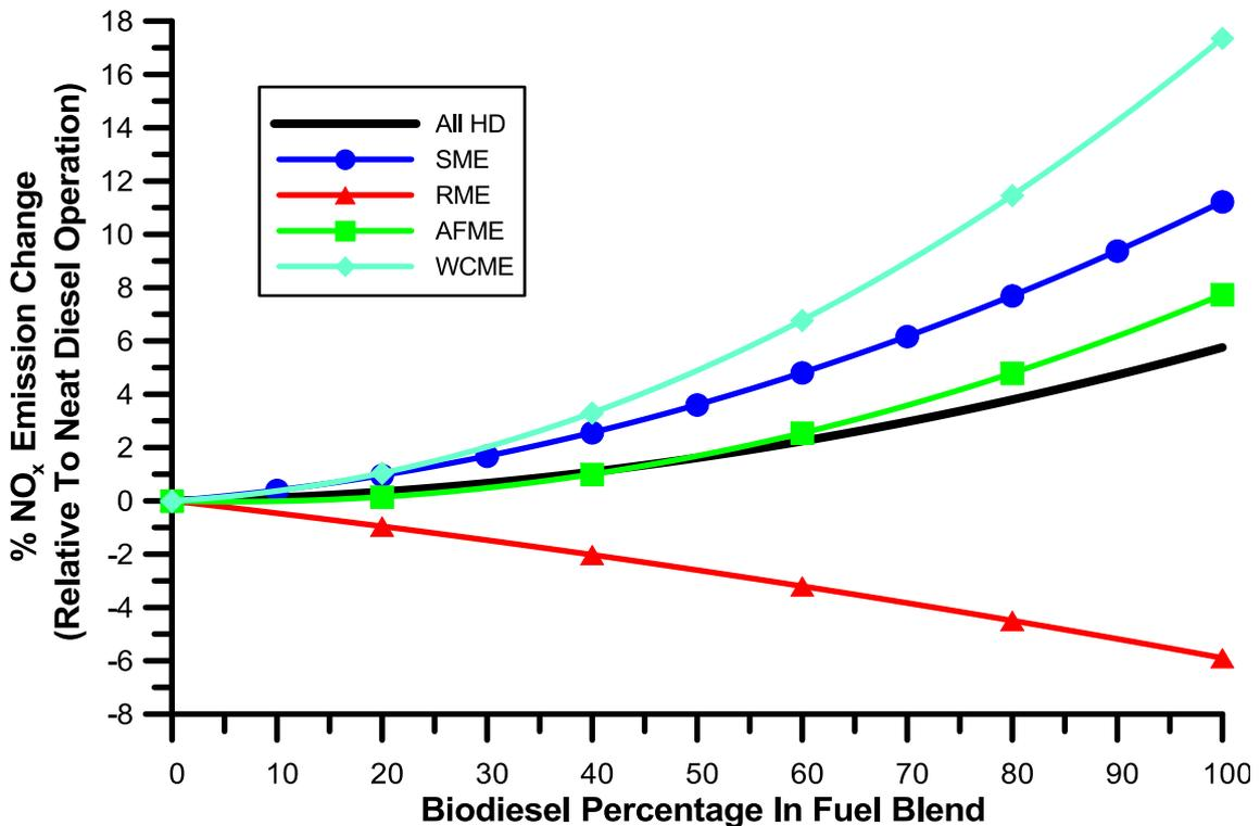
**Fig. 22** – Comparative NO<sub>x</sub> emission change best-fit curves for HD engines and for various biodiesel feedstocks.
