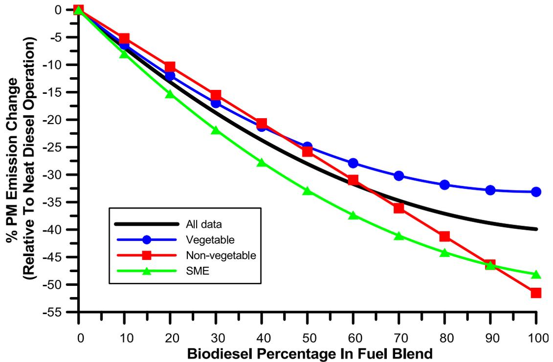
**Fig. 19** – Comparative PM emission change best-fit curves for various biodiesel feedstocks.
