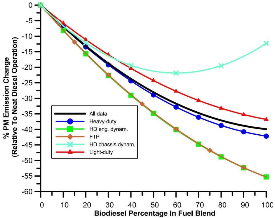
**Fig. 9** – Comparative PM emission change best-fit curves for various transient cycles and engine types.
