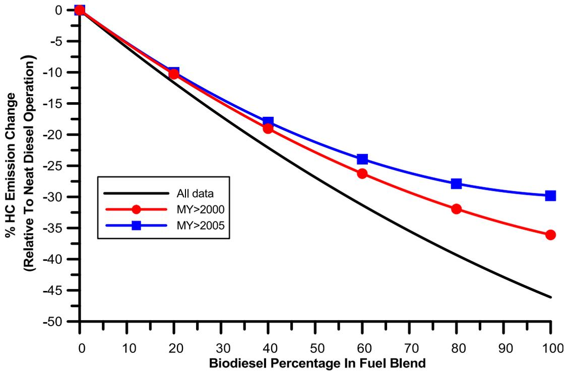
**Fig. 17** – Comparative HC emission change best-fit curves for various engine model years.
