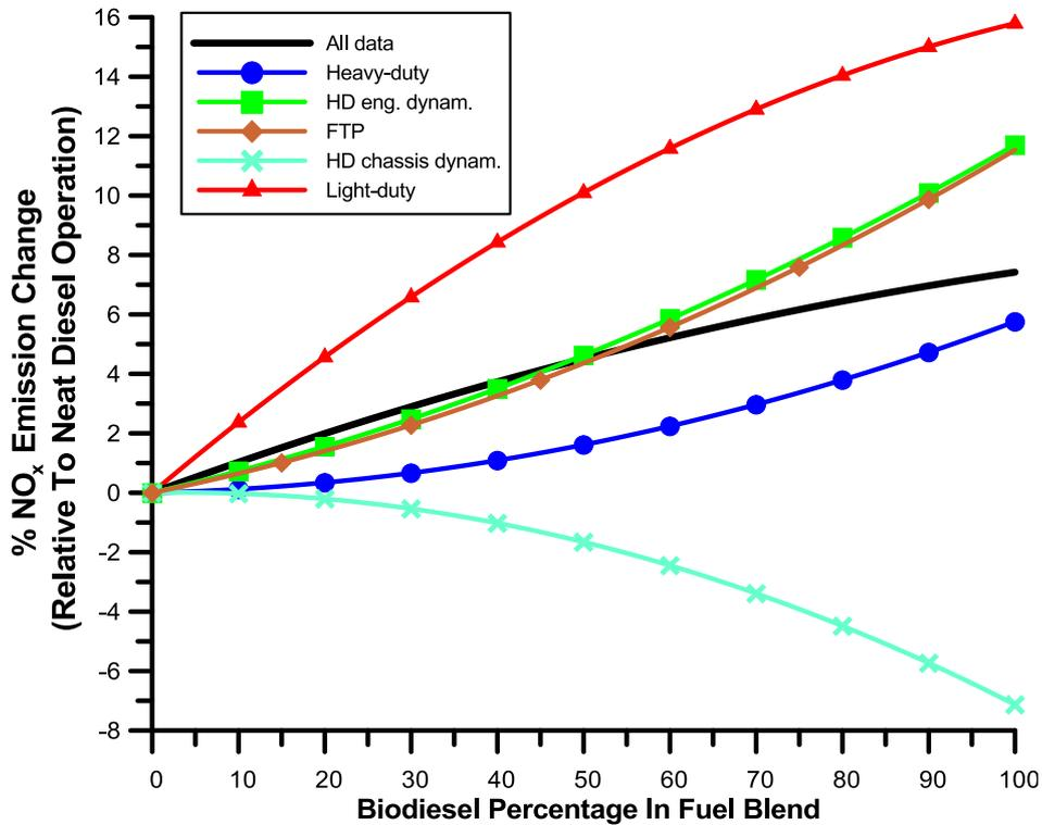
**Fig. 10** – Comparative NO<sub>x</sub> emission change best-fit curves for various transient cycles and engine types.
