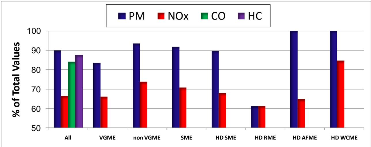
**Fig. 23** – Percentage of total negative (PM, CO, HC) or positive (NO<sub>x</sub>) measurement values for each biodiesel feedstock.
