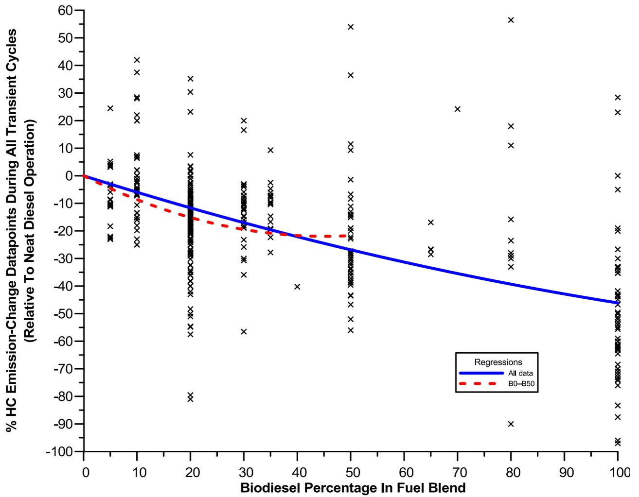
**Fig. 7** – HC emission-change datapoints and best-fit curve when using various biodiesel-diesel blends during all transient cycles.
