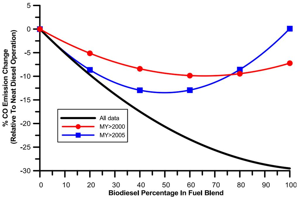
**Fig. 16** – Comparative CO emission change best-fit curves for various engine model years.
