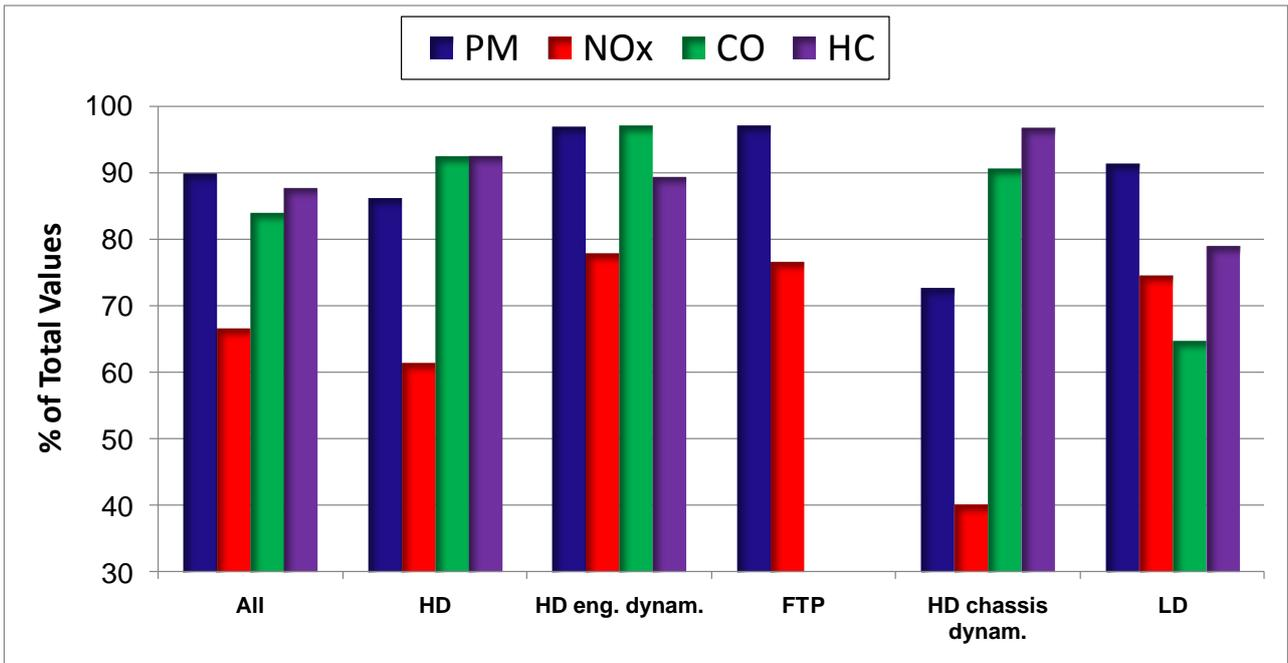
**Fig. 13** – Percentage of total negative (PM, CO, HC) or positive (NO<sub>x</sub>) measurement values for each engine cycle and engine type.
