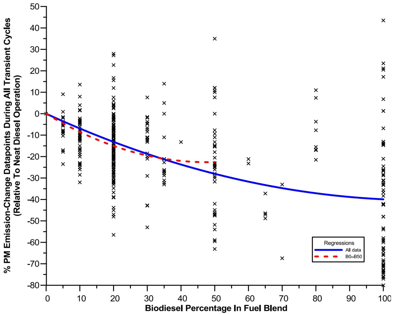
Fig. 4 – PM emission-change datapoints and best-fit curves when using various biodiesel-diesel blends during all transient cycles.
